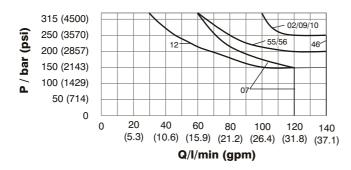
This functional limits have been obtained with warm solenoid condition and at 10 undervoltage from the selected nominal value. All flow data given is considered for 2 flow directions (eg. P to A and simultaneously from B to T). For single flow direction only (4-Way-Valve used as a 3-Way-Valve) the permissible flow must be reduced by as much as 25....30 in comparison to the data shown.
