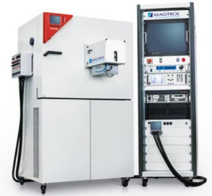
System for certification of automotive electric motors in specific climatic conditions
