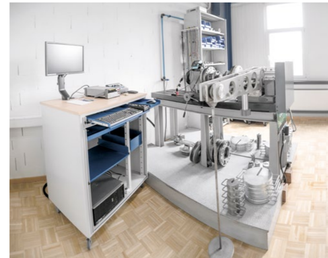
20... 5000 N·m Frictionless Calibration System using double lever and calibrated weights.
