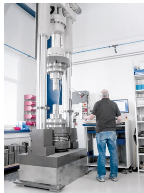
Configuration for rotating torque sensors measurement
