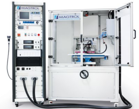
System with multiple lines to facilitate the testing of different devices with the same installation
